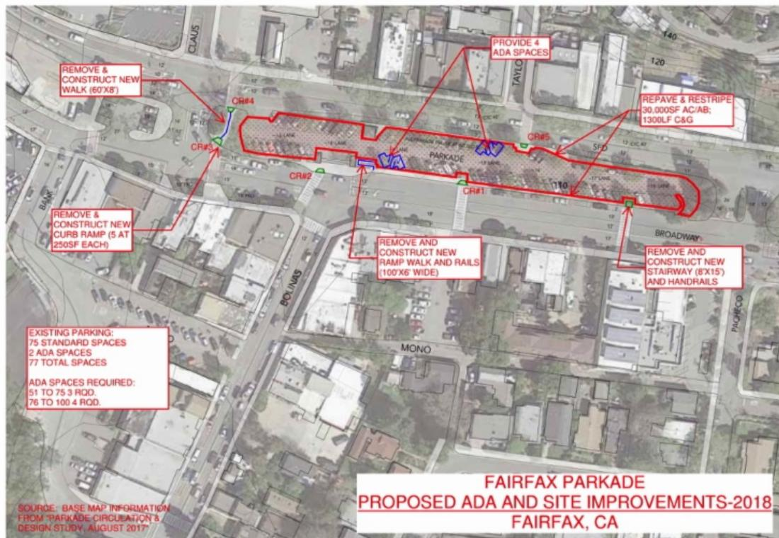
*Existing Conditions.* Line work indicates existing features, such as sidewalks, traffic lanes, curb lines, parking stalls, and building edges. Below the line work, an aerial photograph adds information. Design work was performed using available site mapping. A reliable survey should be obtained prior to more detailed design development.
